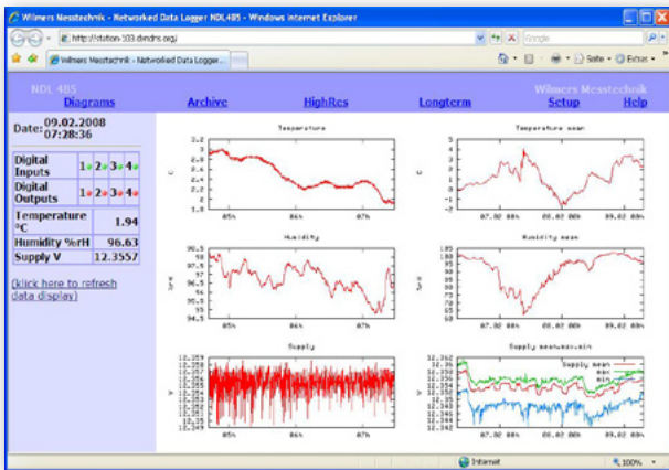
Internet access to an NDL 485 research via DynDNS from a desktop PC
